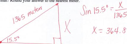
The upper terminal is 365 meters above the lower terminal.
