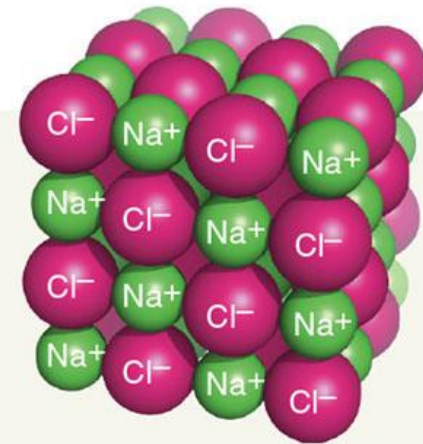
A A crystal of table salt is a cubic lattice of many sodium and chloride ions.
